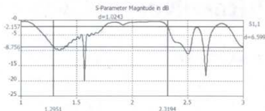
Fig. 16 Return Loss 1 to 3 GHz
